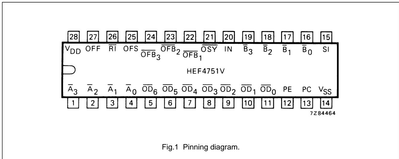
Fig.1 Pinning diagram.
